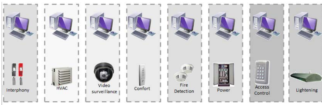
Fig 1.: Several supervision systems running in parallel
