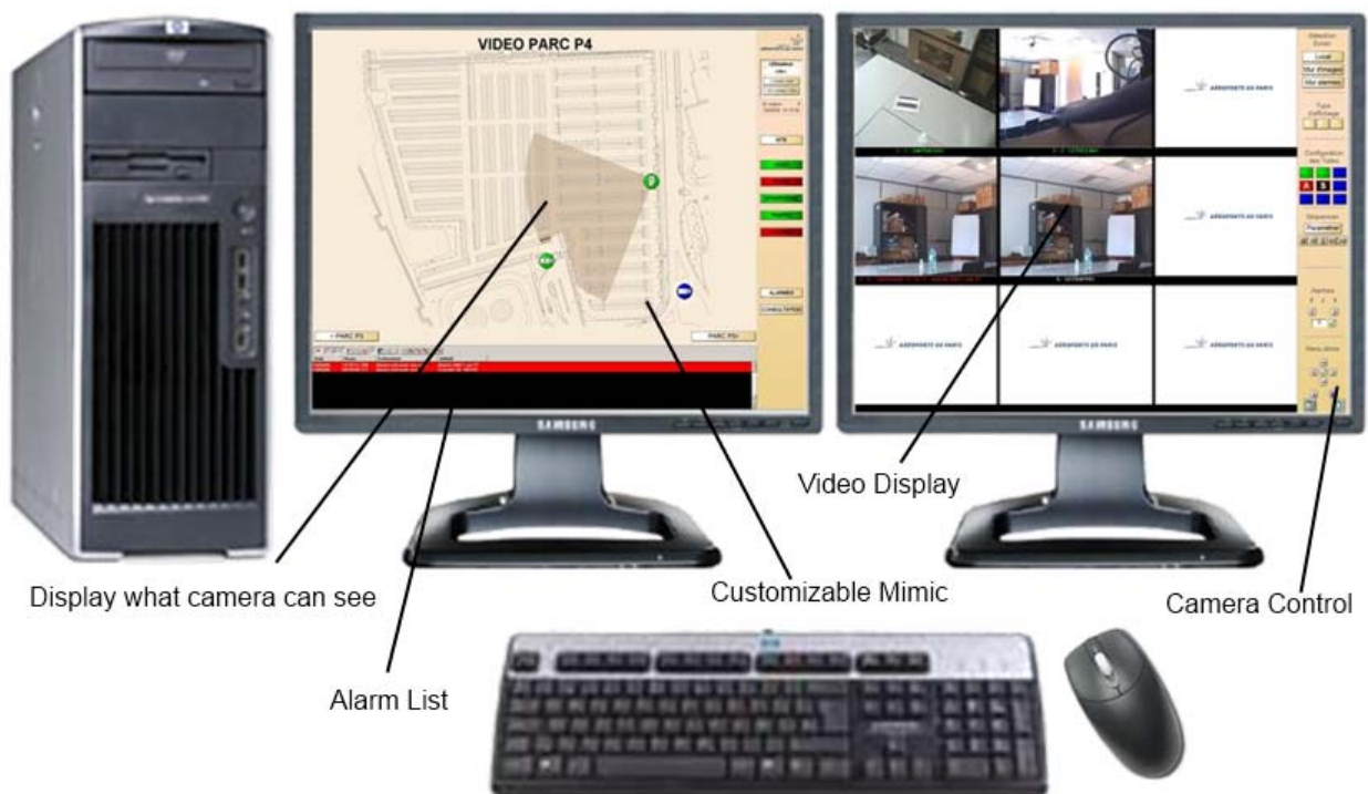
Fig 3: Video integration in Building Management System
