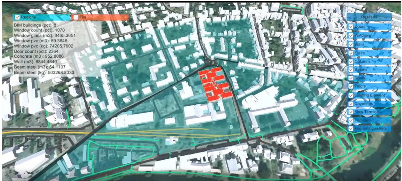
Figure 11. Parcel-based BIM-GIS queries to filter recyclable materials in case these areas are decided to be demolished or transformed
