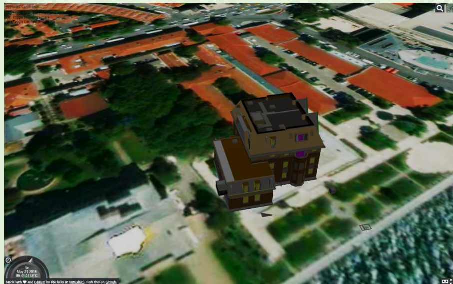
Figure 7 Screenshot on viewing the Schependomlaan BIM model (openBIMstandards, 2015) on a Cesium based web viewer
