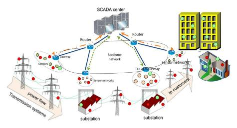
A typical Wireless Sensor Networks based Smart Grid
