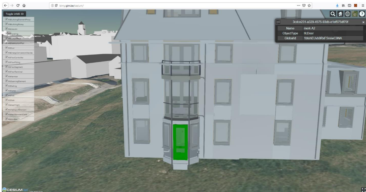
Figure 19 Screenshot of a simple Web application that visualizes 3D Tiles of the Schependomlaan IFC (openBIMstandards, 2014)
