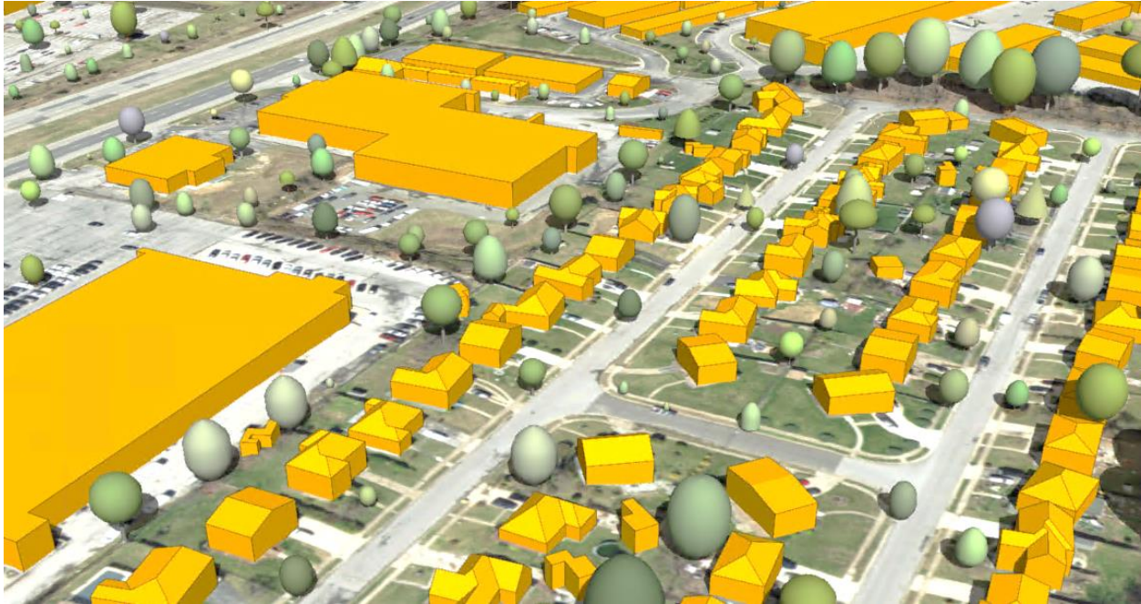
Figure 27 Extraction of trees from LiDAR point clouds
