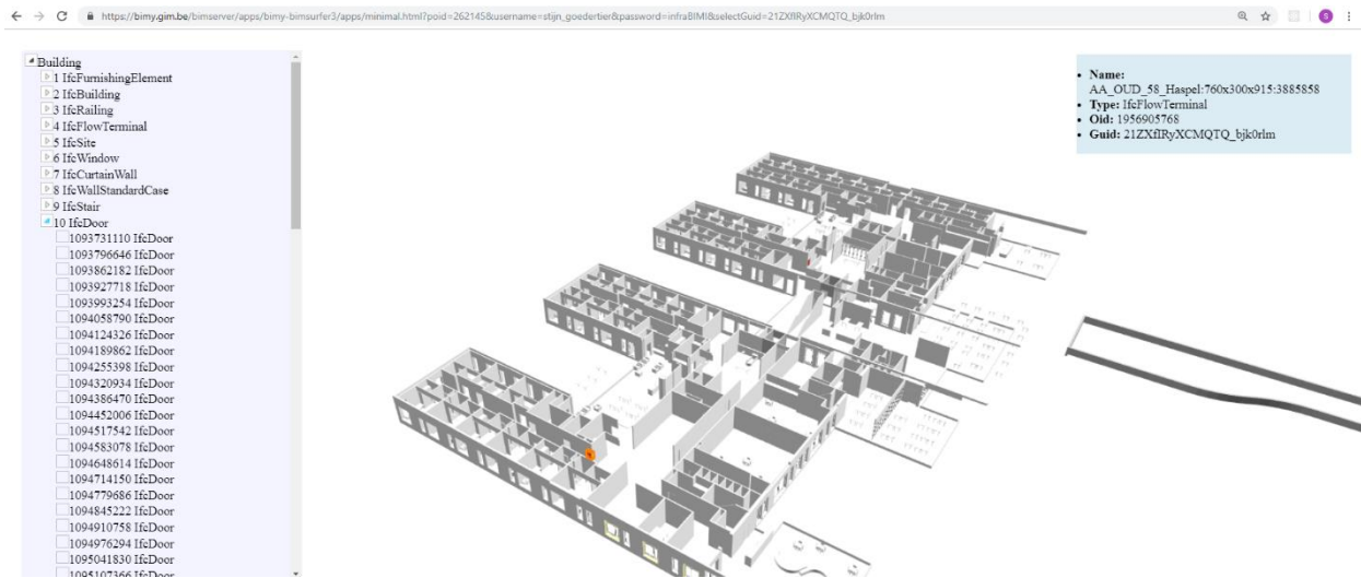
Figure 14 IFC to 3D IFC floorplan visualized with BIMsurfer3 (ASSAR, 2019)
