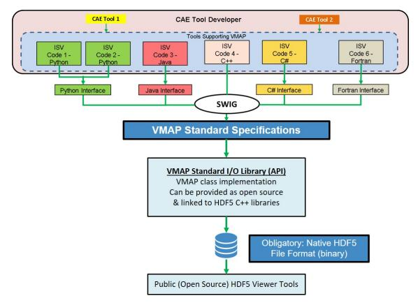
Figure 5.2: Extended VMAP Software Architecture
