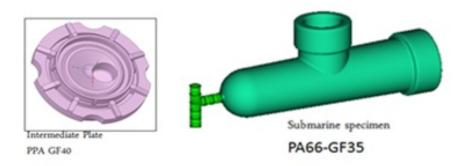
Figure 6.9: Injection moulded Components - Fatigue
