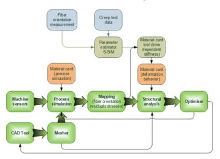
Figure 6.11: Simulation process workflow - Injection Moulding - Creep
