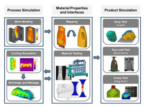
Figure 6.2: Simulation process workflows - Blowforming
