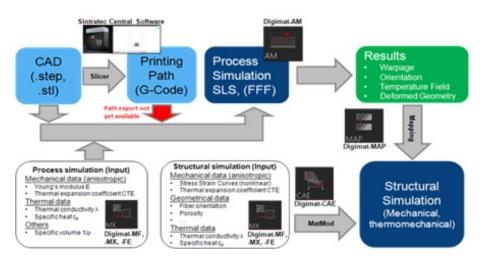
Figure 6.13: Simulation process workflow - Additive Manufacturing
