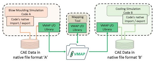
Figure 5.3: VMAP Standard API in CAE chain simulation process
