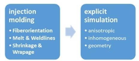
Figure 6.6: Simulation process workflow - Injection Moulding - Impact
