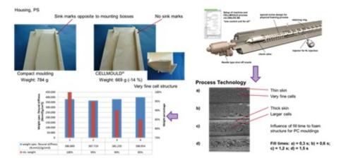
Figure 6.7: Injection Moulded Parts - Foaming
