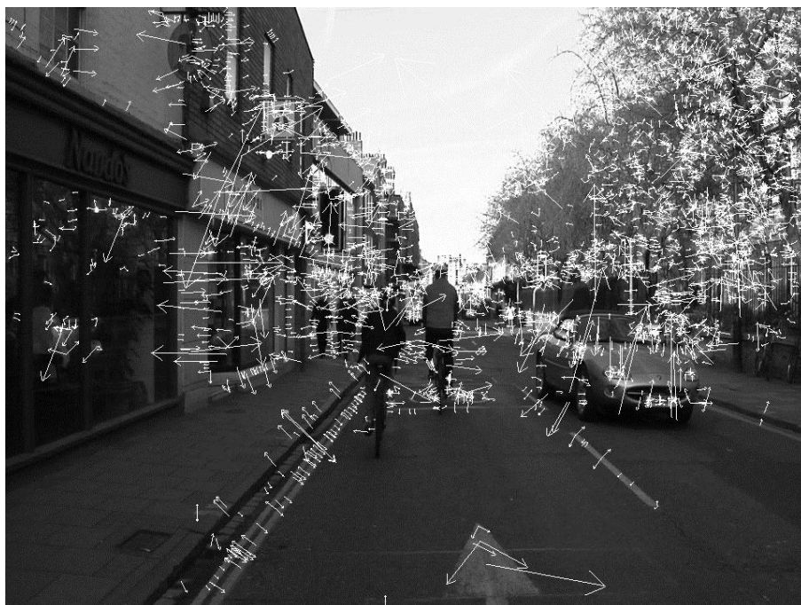
Figure 8: The SIFT salient points. The salient point is located at the origin of the arrow; the length of the arrow represents the scale, its direction the argument of the gradient.
