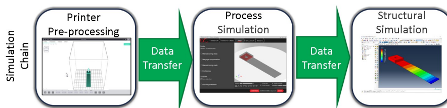
Figure 5.6: Simulation process workflow.
