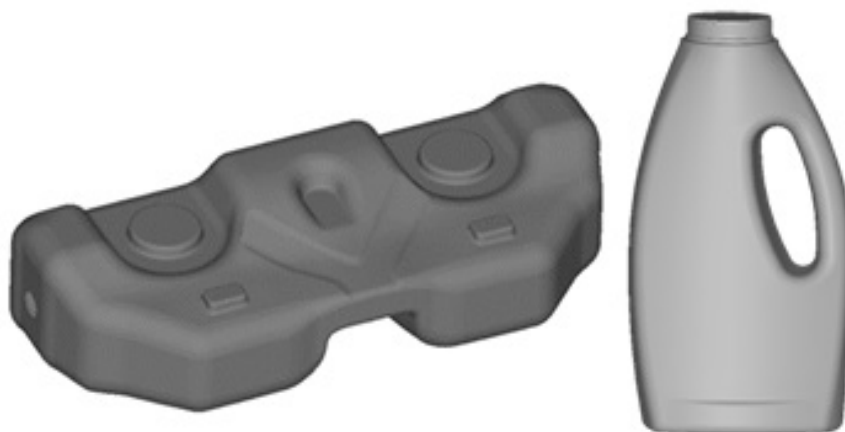
Figure 5.1: Examples of blow moulded components.
