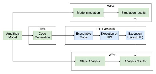
Figure 2.15: RTFParallella in connection to other work packages in Panorama
