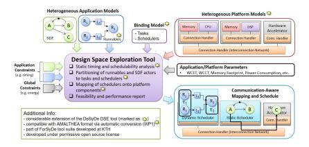
Figure 2.7: KTH view of DSE for heteroegeneous systems
