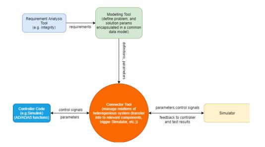
Figure 2.1: High level architecture for demonstrator use case
