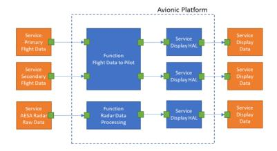
Figure 2.9: Functional break-down at functional abstraction level
