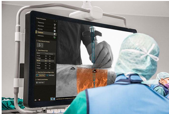
Figure 26 AR in spine surgery. External view of the patient is combined with X-ray images of the spine and device tracking and path prediction and displayed on a big screen
