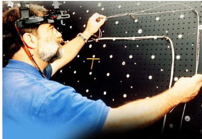
Figure 19 Augmented reality system introduced in 1990 in Boeing to help technicians to wire different plane's boards
