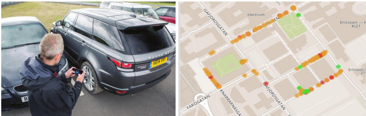
Figure 17 (a) Direct teleoperation from Jaguar-Land-Rover group. (b) Feasibility of using cellular network for direct teleoperation from Ericsson.
