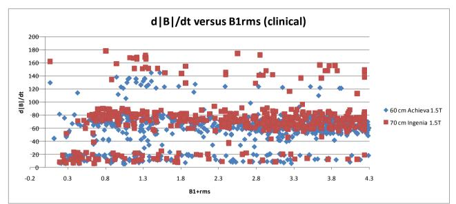
Figure 5. Scatter plot of calculated d|B|/dt values versus  $B_1^+_{RMS}$  for factory clinical sequences delivered with 60 cm and 70 cm MR systems. The orange dotted line indicates the allowed range of sequence parameters. A significant number of protocols (esp. TSE and bFFE), running in 1<sup>st</sup> level controlled mode, are (obviously) excluded by FPO, and need re-evaluation.
