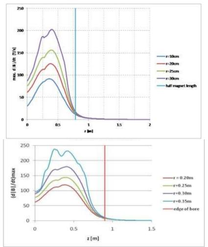
Figure 1. Graphs showing the maximum d|B|/dt at different radii around the central line of the bore of the MR system, for 60 cm, 40 mT/m, 200 T/m/s (top), and for 70 cm, 33 mT/m, 200 T/m/s (bottom).
