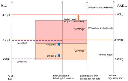
Figure 4. Schematic representation of (1.5T)  $B_{1rms}$  values and corresponding WB SAR values for typical body coil designs. Reported 2W/kg may results in significantly different actual deposited powers for different systems. Further margins may be applied by MR manufacturers to account for e.g.  $B_1^-$  contributions. Body Coil designs affect the conversion between  $B_{1rms}$  and WB SAR.
