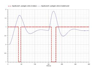
Figure 6: Requirement Req 002 status for tank 1 in the overflow scenario
