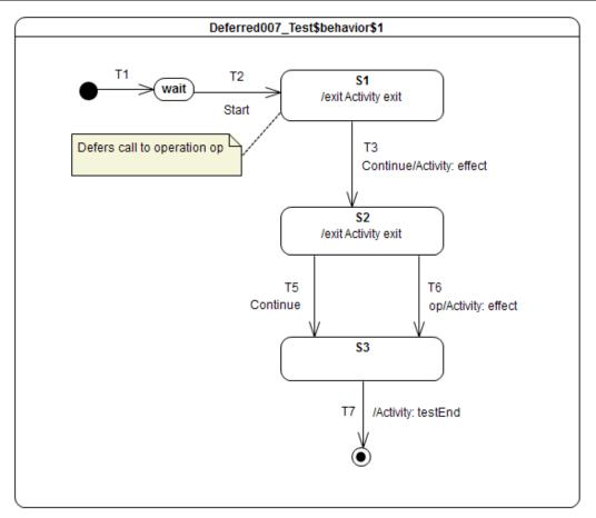
In this test, the call event occurrence corresponding to the op operation is dispatched when in configuration S1. This implies the state machine accepts and defers the event occurrence. At the end of the RTC step, the tester (i.e., the object that emitted the call) shall remain suspended. This shall be maintained until the end of the RTC in which the transition T6 is fired. To demonstrate this semantics, Deferred007 Test shall be refactored.
