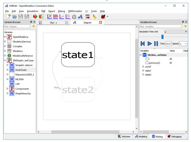
Figure 4. State machine debugger in OMEdit.
