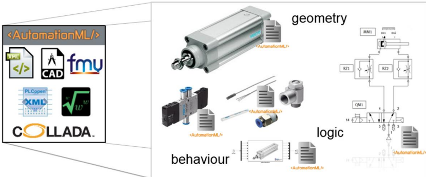
Figure 23: Container format for a pneumatic drive
