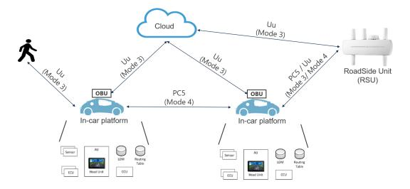
Figure 3.36.: V2X Cellular communication for the communication types of Figure 3.20
