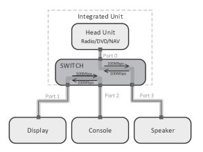
Figure 3.18.: Automotive Ethernet
