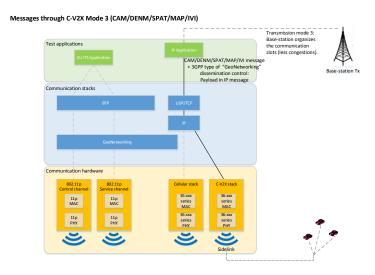
Figure 3.25.: Message communication through Cellular-V2X Mode 3
