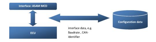
Figure 3.19.: Interface to the ECUs (for MC-Application) [5]
