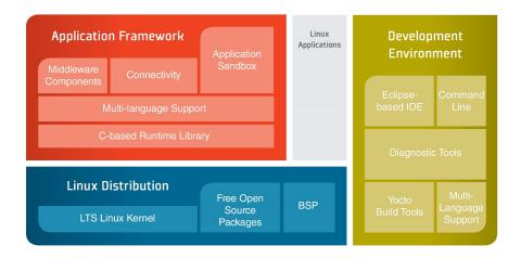
Figure 3.2.: Legato Software Architecture [135]
