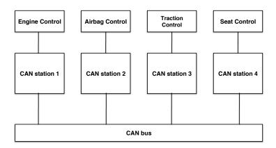
Figure 3.11.: CAN system example
