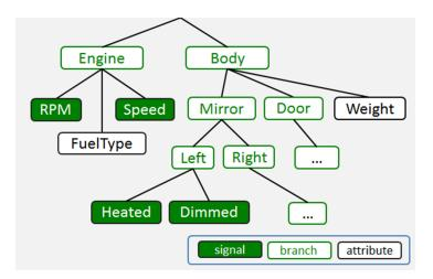
Figure 3.7.: An excerpt of the Vehicle Signal Specification [77]
