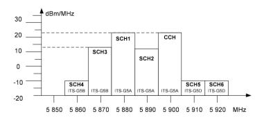
Figure 3.32.: Maximum mean spectral power per channel
