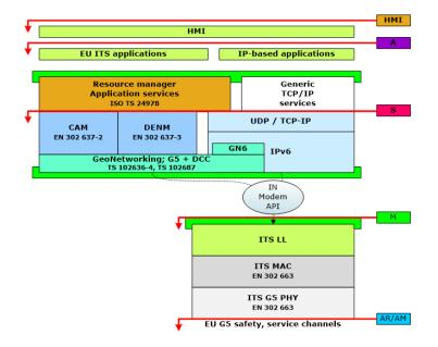
Figure 3.29.: Deployment of software on the 11p hardware
