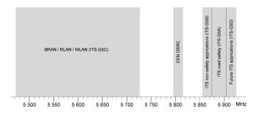
Figure 3.30.: Overview of channel types allocated for the 5 GHz frequency range
