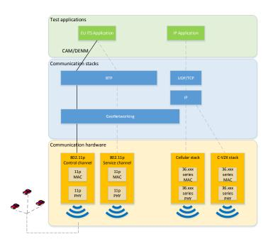
Figure 3.21.: ETSI safety message communication through 802.11p
