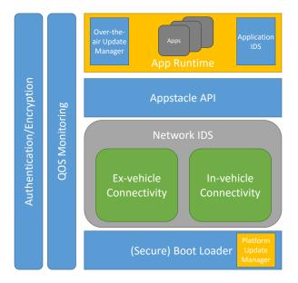
Figure 1.1.: The logical architecture of the APPSTACLE in-vehicle platform
