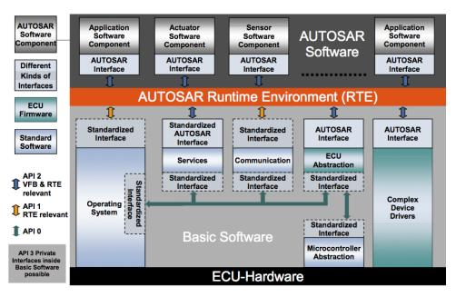
Figure 3.6.: The AUTOSAR Layer Model [11]
