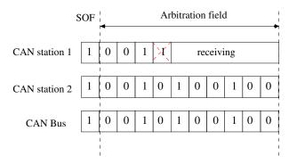
Figure 3.12.: CAN arbitration mechanism
