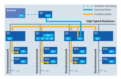
Figure 3.49.: Overview of ECU network in high-end vehicles [43]
