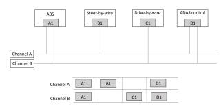
Figure 3.15.: FlexRay Static Segment
