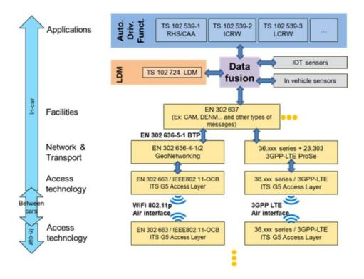
Figure 5.2.: Conceptual architecture of V2X communication channels in ITS
