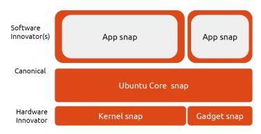
Figure 3.3.: Ubuntu Core Software Architecture [160]
