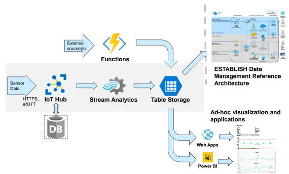
Figure 27. The reference implementation for environmental data collection and processing in the Finnish pilot.
