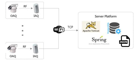
Figure 19. Basic technical requirement of intelligent air quality management system.
