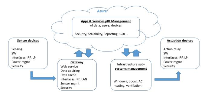
Figure 16. High-level component specification on the HVAC use case.
