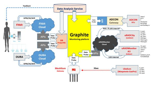
Figure 4. Sensors Architecture.
