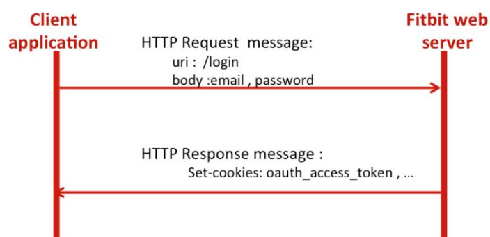
Figure 9: Medolution Device Connector instantiation for FitBit devices: session initiation
