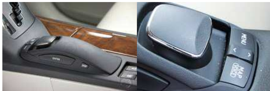
Figure 3-26 Lexus RX450h Force Feedback Enhances Driver Experience and Safety IMMERSION
