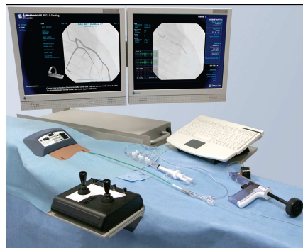
Figure 3-23 The AccuTouch system *graphics and forcefeedback action IMMERSION
