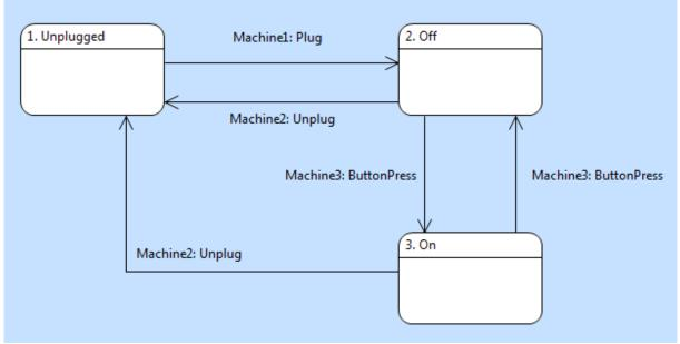
Figure 16 - An xtUML State Machine
