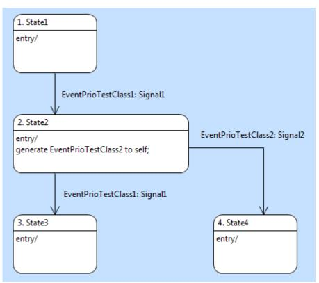
Figure 20 - State Machine with Self Event
