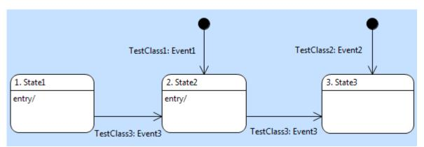
Figure 17 - State Machine with Creation Transitions
