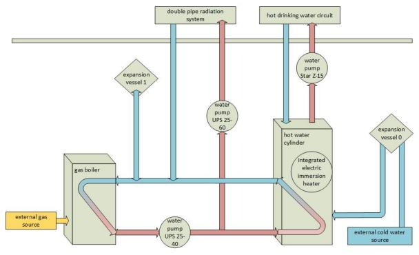
Figure 4-10: Overview of a Heating Circuit.
