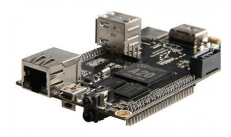
Figure 57: Singe-board computer Cubieboard2
