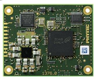
Figure 58: System on Module phyCORE-OMAP5430
