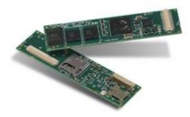
Figure 51: Mainboard Gumstix Verdex Pro 6LP and Ethernet interface board Netpro-vx
