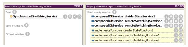
Figure 38: Definition of the SynchronizedSwitchingService
