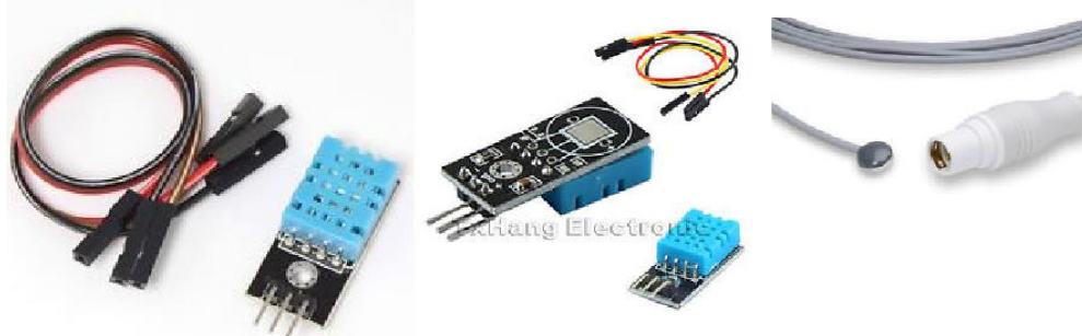
Figure 31: Examples of skin humidity and temperature sensors
