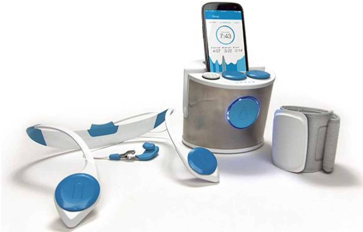
Figure 15: VITALITI system (recording of ECG, heart rate...)
