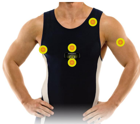
Figure 22 Ambiotex t-shirt with integrated sensors
