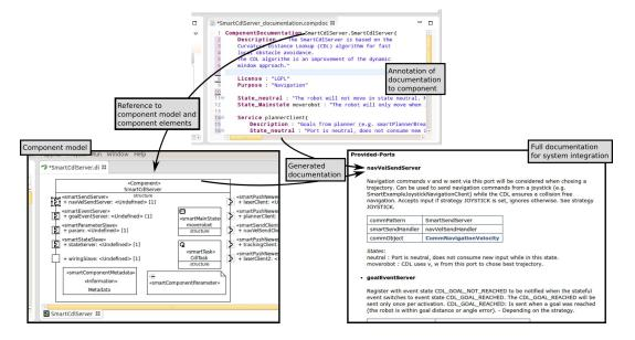
Figure 2.25. Information from the documentation and component model is transformed to a complete documentation (right) for later system integration which assists the system integrator during composition. [4]
