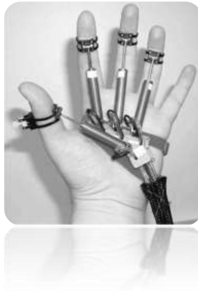
Figure 4: Example of force-feedback glove with pneumatic pistons to simulate grasping (courtesy of Human Machine interface laboratory of Rutgers University)
