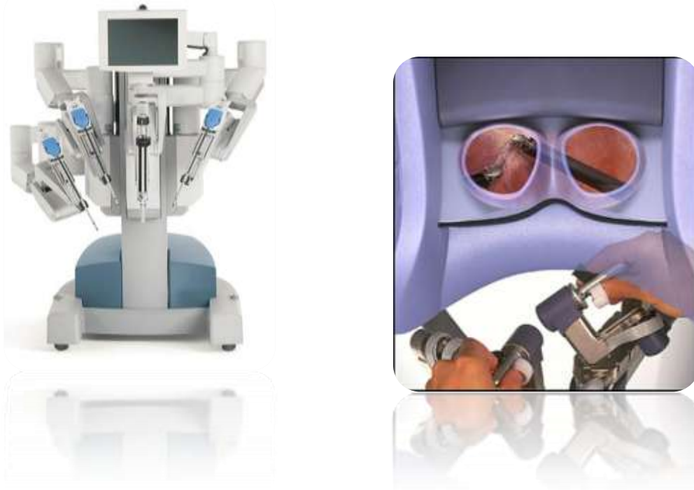
Figure 8: da Vinci surgical system (Intuitive Surgery). It consists of an ergonomic user haptic interface, co-axial hand-eye alignment, stereoscopic viewer, and instruments with seven degrees of freedom, fingertip control of the surgical gestures.
