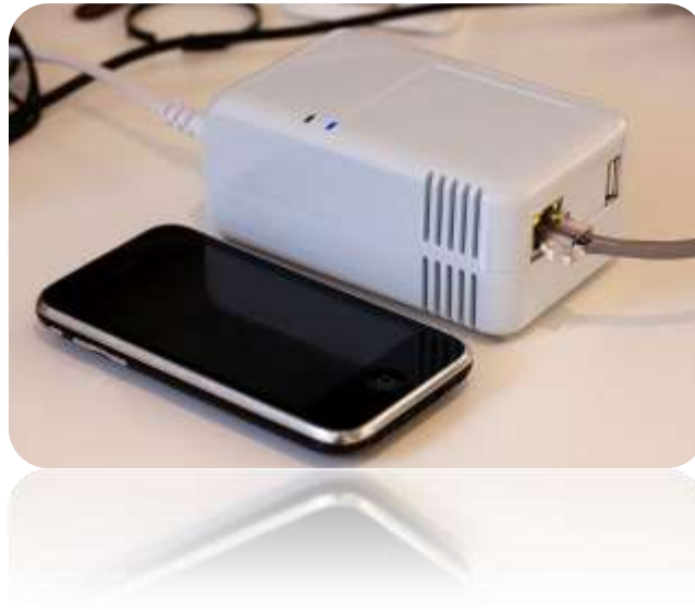
Figure 9: Marvell Technology Group's 11 SheevaPlug plug computer with iPhone (approx 115 mm x 60 mm) for scale
