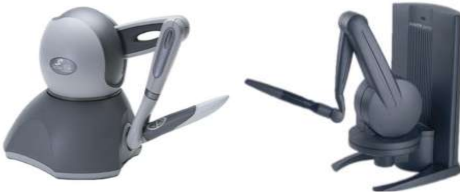
Figure 5: Types of haptic interfaces: Omni ® (left) and phantom Desktop ® (right). Courtesy of Sensable ® Tech.
