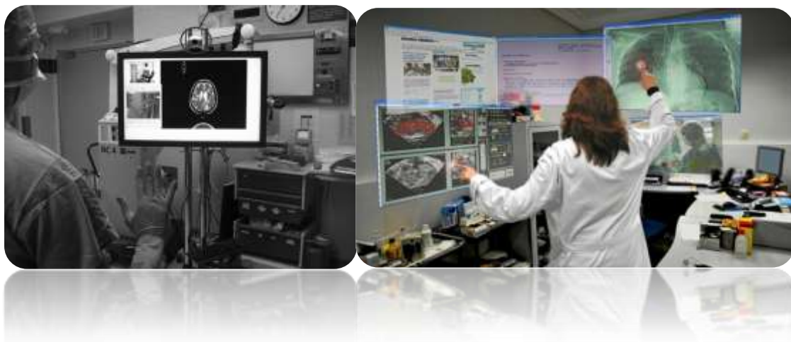
Figure 2: on the left, one example of applied medical research in the field of gesture recognition for browsing of radiology images ( Gestix , (J. P. Wachs et al., 2008)). It is an application based on a real-time hand-tracking recognition technique using color and motion fusion. On the right, an application of gesture recognition expected in the near future.
