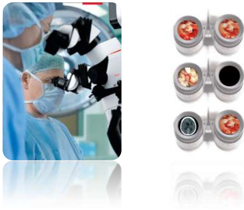
Figure 11: Example of AR for neurosurgical application. The Leica DI C500 is an image injection device for Leica microscopes. Several type of information (i.e. 3D reconstructions, patient preoperative images, etc.) can be visualized inside one of the ocular (image on the right).
