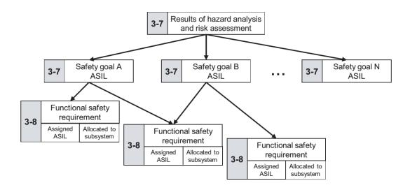
Figure 1.2.: Derivation of Safety Requirements (source: [5])
