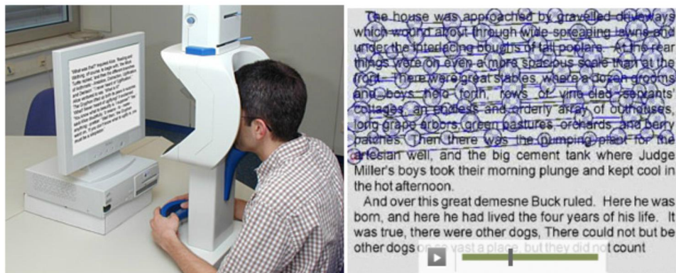
Figure 21. Eye and gaze tracking solutions can assist in monitoring on-screen eye movements in reading, following verbal directions in finding objects, and saccades/anti-saccades based on read or verbal instructions for both the qualitative and quantitative observation of the behavioural areas [smivision2012].
