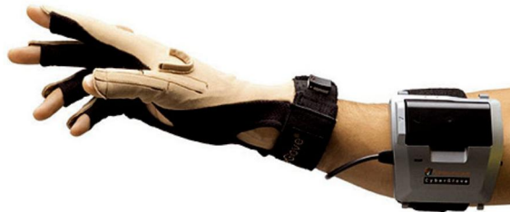
Figure 27 - The CyberGlove from the Immersion Corporation (from [A]).
