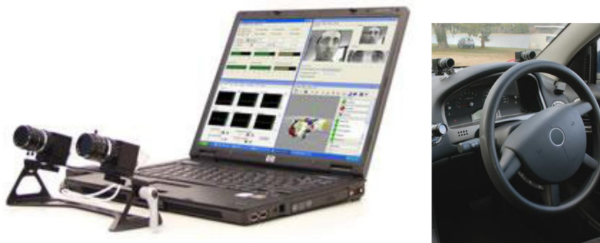
Figure 23. faceLAB is capable of providing head and eye tracking data for research into human behavior in real vehicles, cabins and cockpits, both indoors or outdoors. [facelab2012].
