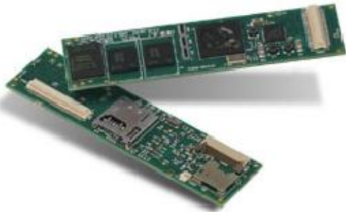
Figure 45: Mainboard Gumstix Verdex Pro 6LP and Ethernet interface board Netpro-vx
