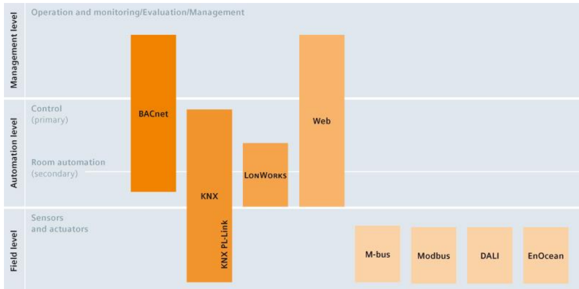
Figure 6: Communications protocols as used in the different levels of the automation pyramid [9]
