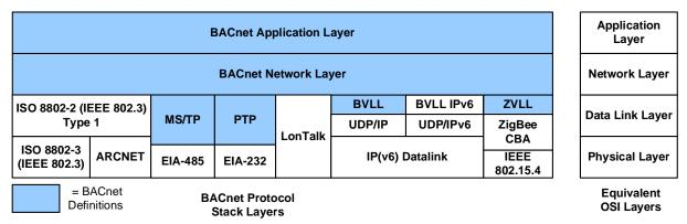
Figure 16: Collapsed BACnet Architecture.
