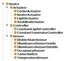
Figure 31: Example Classification of Building Equipment
