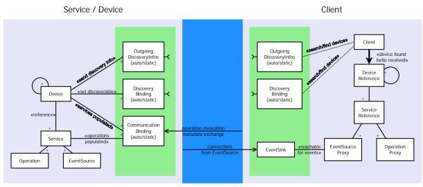
Figure 9: JMEDS frame structure
