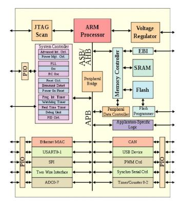
Figure 44: Block diagram of SoC
