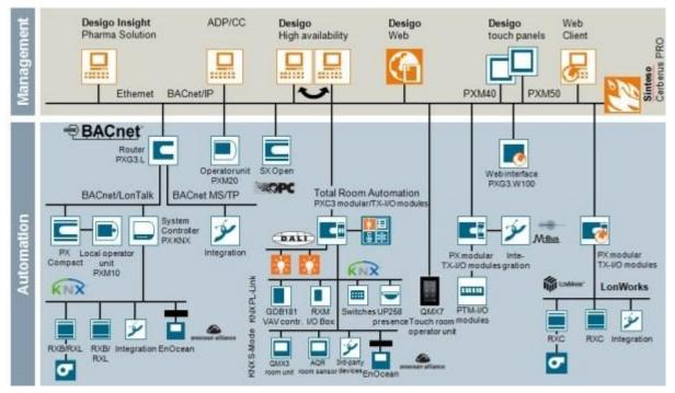
Figure 5: System topology of DESIGO BAS from Siemens [7]
