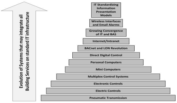
Figure 1: Evolution of Building Automation and Control Systems [3]
