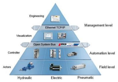
Figure 2: Automation pyramid (Source: Rexroth, Bosch Group)
