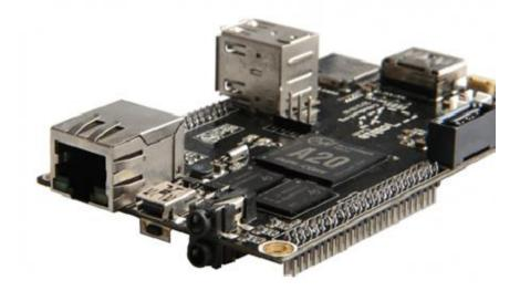
Figure 51: Singe-board computer Cubieboard2
