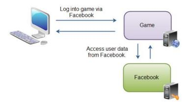
Figure 10: Example of how OAuth 2.0 is used (from [91])
