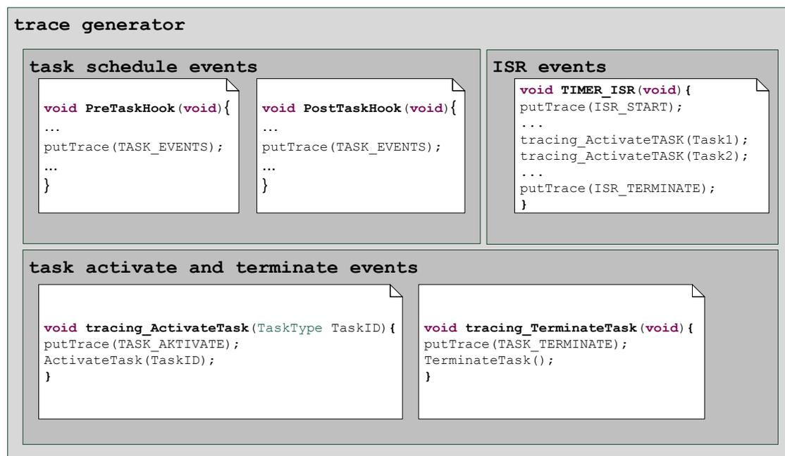
Figure 9.1: HTF trace generator in the embedded trace concept
