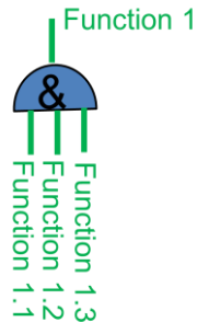
Figure 20: Functional perspective presentation C Function 1 represents the sequential interaction of the 3 sub-functions.
