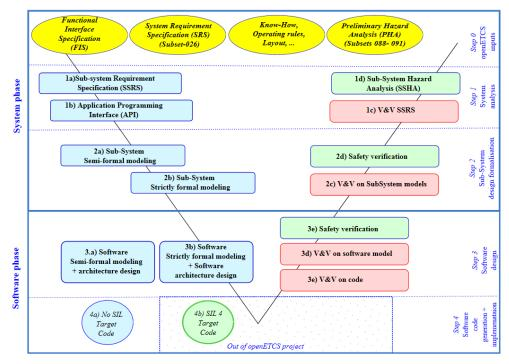
Figure 1. openETCS Process (rough view)
