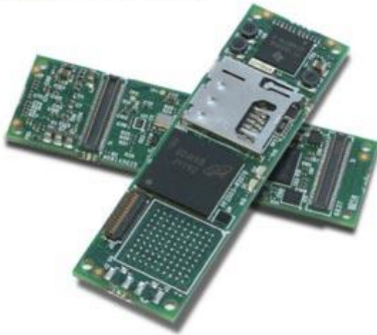
Figure 6.17: Computer Gumstix Overo Earth.
