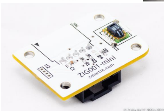
Figure 6.10: Different images of the Zolertia WSN motes
