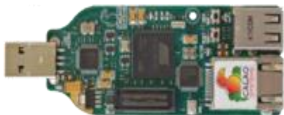
Figure 6.18: One-board computer CALAO USB-A9G20-C01.
