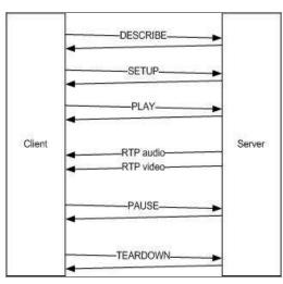
Figure 4: RTSP communication between server and client
