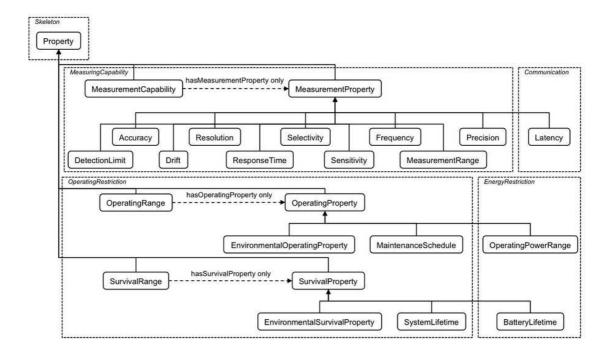
Figure: Enumeration of the measurement, environmental and survival properties [3].
