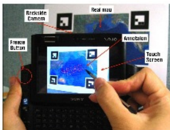
Figure 59: Prototype implementation: annotating on a real map
