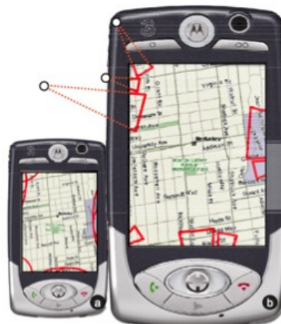
Figure 38: (a) The problem: Halo arcs point users to off-screen targets, but overlapping arcs are hard to interpret. (b) Wedges point to the same off-screen locations; since they avoid overlap, the display remains intelligible
