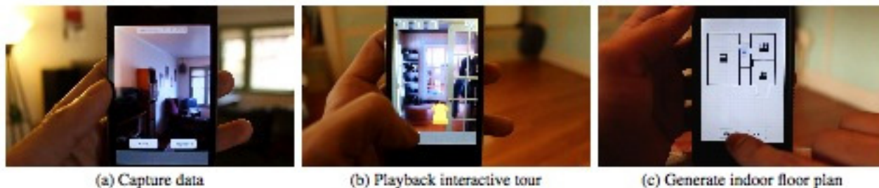
Figure 56: The proposed system captures an interactive visual tour and a floor plan of an indoor scene, in real time, on a smartphone. (a): Capture data; (b): Playback interactive tour; (c): Generate indoor floor plan
