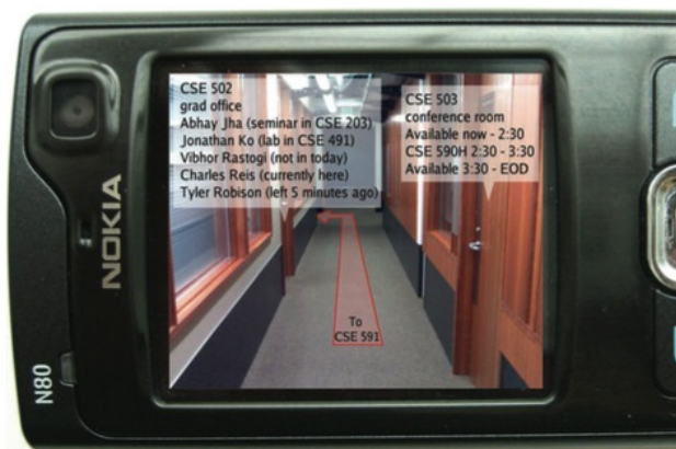
Figure 52: Information overlays on a camera-phone display image. The image shows both an overlaid navigation aid (the directional arrow) and a “magic lens” type window for displaying dynamic information about the current surroundings
