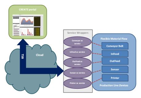
Figure 3: Devices as web services in the demonstrator
