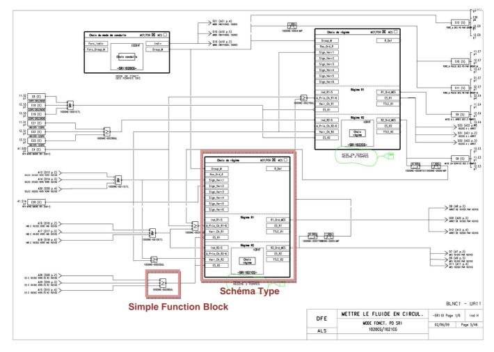
Figure 3 : Example of a Functional Diagram (DFE) for EDF I&C system
