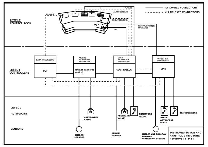
Figure 1 : Illustration of the I&C System of a 1300 MW nuclear power plant
