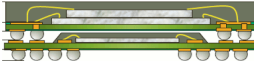
Figure 46 - Package-on-package, with processor, flash and RAM
