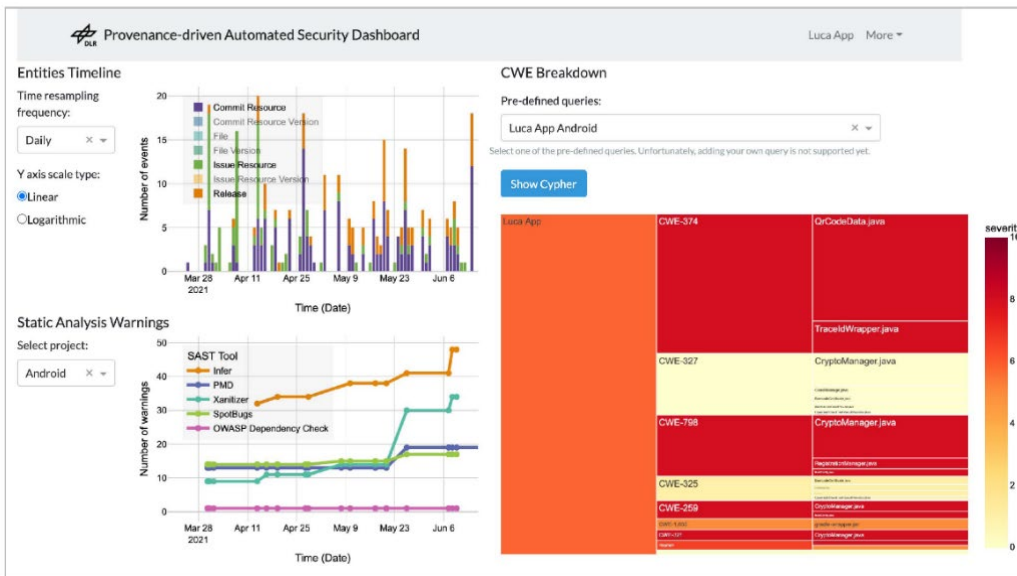
Figure 40. Interactive visualization dashboard which provides an overview of security analysis results from multiple SAST tools based on the provenance information of the code base [21].
