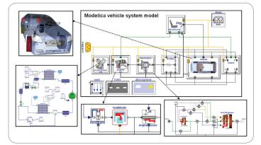
Systems modelling involves the behavioural and dynamic modelling of systems in any engineering domain including control systems, such as the overall model of a vehicle consisting of vehicle dynamics, combustion engine, transmission, drive line, brake and control systems.
